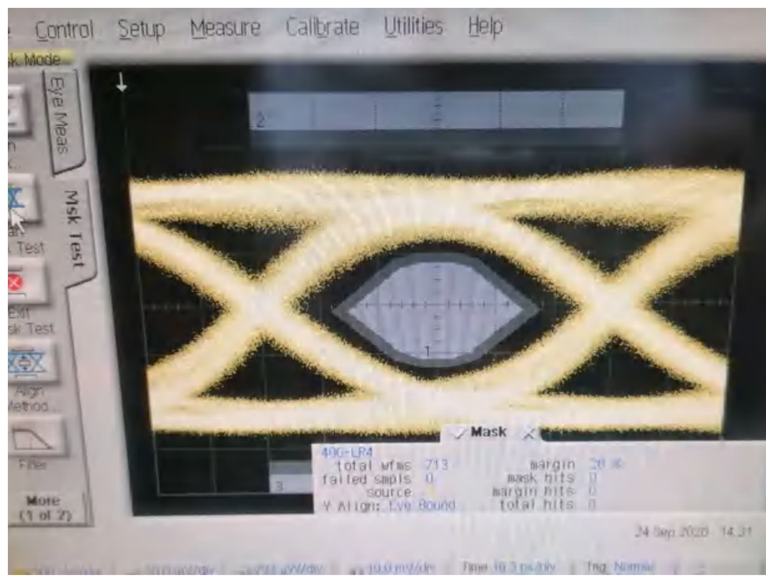
Eye diagram and spectrum at -40°C
